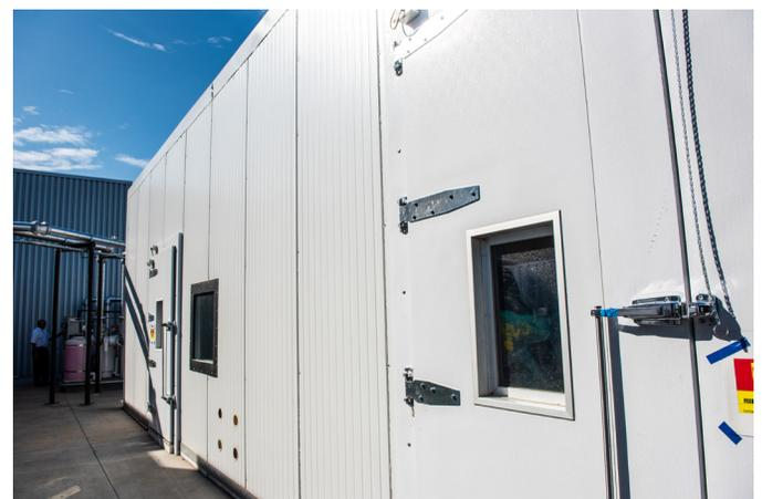
The side-by-side environmental chambers offer respective indoor and outdoor simulation capabilities.
